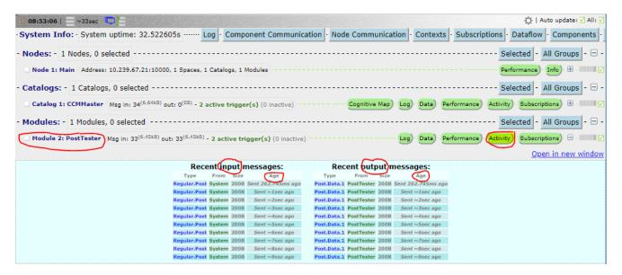
In this example we see a system with two components; one Catalog (called CCMMaster) and one Module (called PostTester). When we click the Activity tab for the module we see the 10 most recent input messages and the 10 most recent output messages. This list will continuously update itself unless you untick the Auto update box for either the module itself (green tick to the far right) or for all (the green tick marked All in the top right corner).
